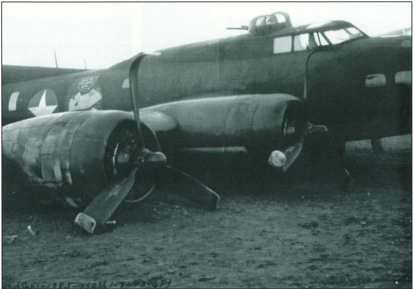
Aircraft accident January 8, 1943. Right main landing gear drag link failure caused gear to collapse during Lt. Donald J. Stoeger's fourth touch-and-go landing. (Courtesy of J. Stoeger)
